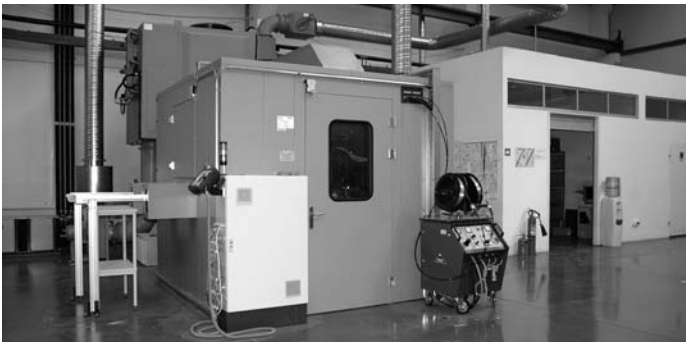
Fig.2 System for metallization of varistors
