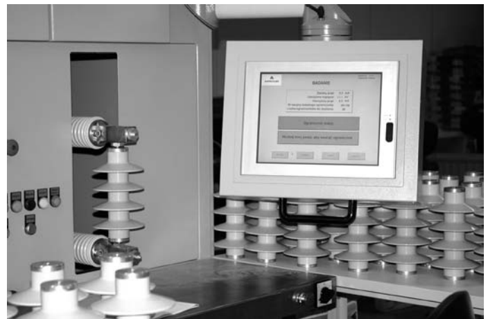
Fig.5 Stand for tests of ASM surge arresters
